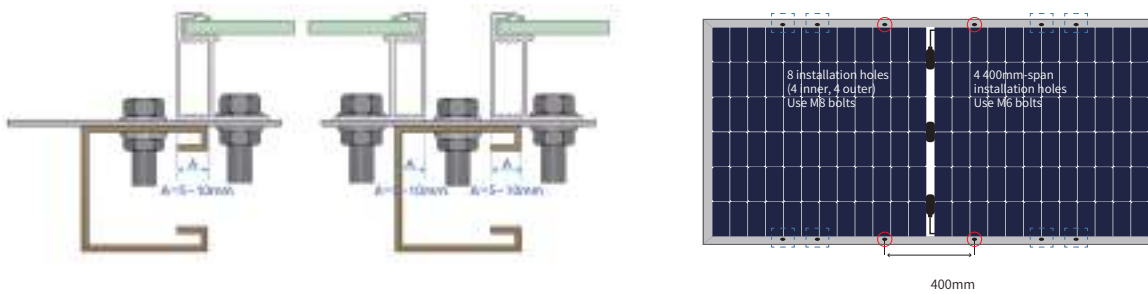
Figure 7 Bolt Installation of Bifacial Module
